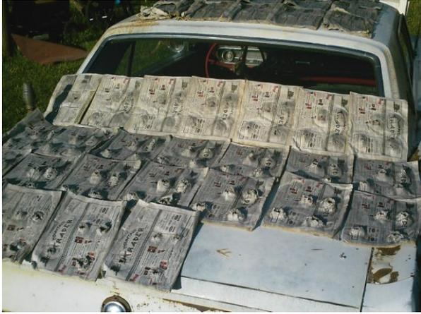
then buried itself in the first few layers of the second bunk of wet newspaper. The other three slugs were found in the last layer of the first bunk bulging out the backside of the bunk.
