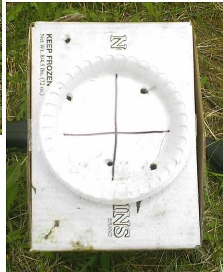
With this particular load combination, which was not a maximum power load, the average penetration depth of the slugs in wet newspaper was 6 inches. One of the slugs penetrated all the way through the first 6" bunk of newspaper, penetrated the plastic bag membrane, and
