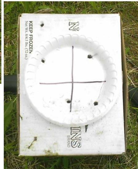
he group as seen is not a single pattern. The two shots on the right were fired from the test gun with a cylinder choke tube in place and the three shots to the left were fired with the full choke tube in place. What you are seeing is mainly vertical stringing which was a problem I was having back then with the particular load combination I was using. The upper left had shot is the one which passed above the test medium.
