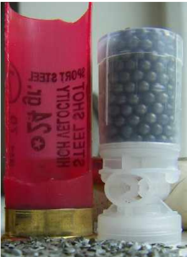
Picture 4. Steel shot pellets are many times harder than lead and possess a degree of elasticity that makes them nigh on perfect for 'Bounce' phenomena to occur.
