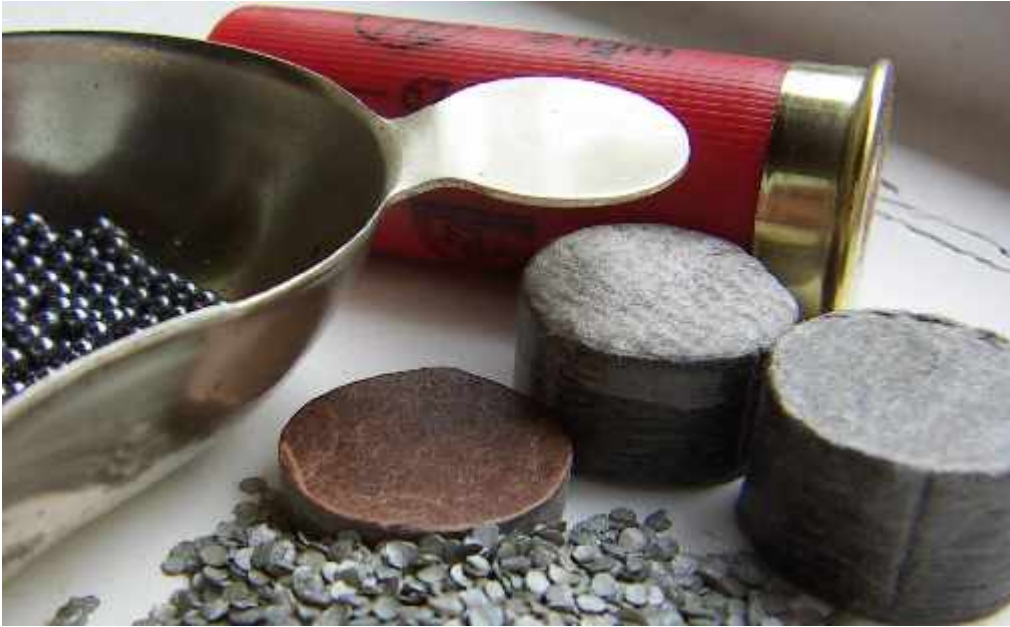
Picture 3. The lead shot used in club fibre wadded loads has very limited 'Bounce' capability.
