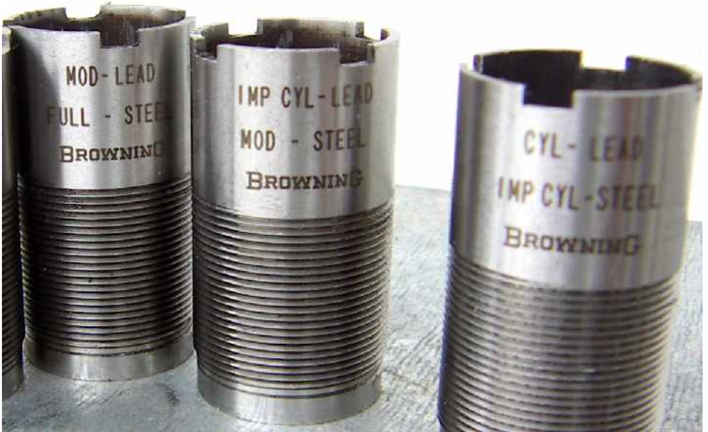
Picture 6. A Modified choke for Lead shot (Half in the UK) is the maximum recommended for steel shot (giving a Full choke pattern), but as clearly indicated, greater degrees of choke are simply not needed with steel pellets. The CYL- LEAD (true cylinder) choke throws around a USA Imp/Cyl (UK quarter choke pattern) with steel shot.
