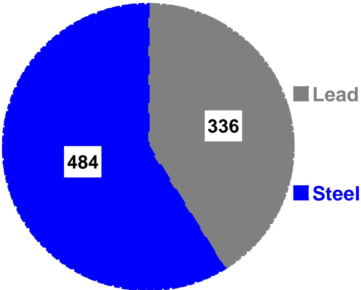
example, then a 28gram loading of 'steel' shot will contain 484 pellets. This same weight of shot in a budget lead loading will have around 336 pellets.
