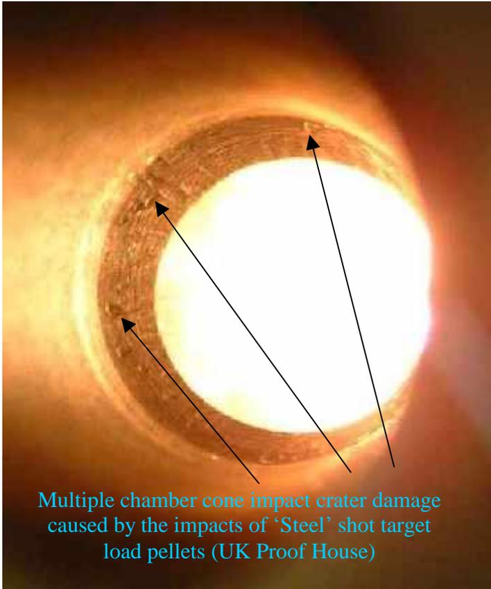
It must be appreciated that the 'Steel' pellets are very much harder than lead, needing mandatory protection of the gun's bores from any contact with them.
