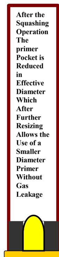
***NB This special treatment of hulls to reduce the primer pocket size is essential when using a self-loader or pump action .410 to prevent possible displacement of the smaller sized primer after firing.***
